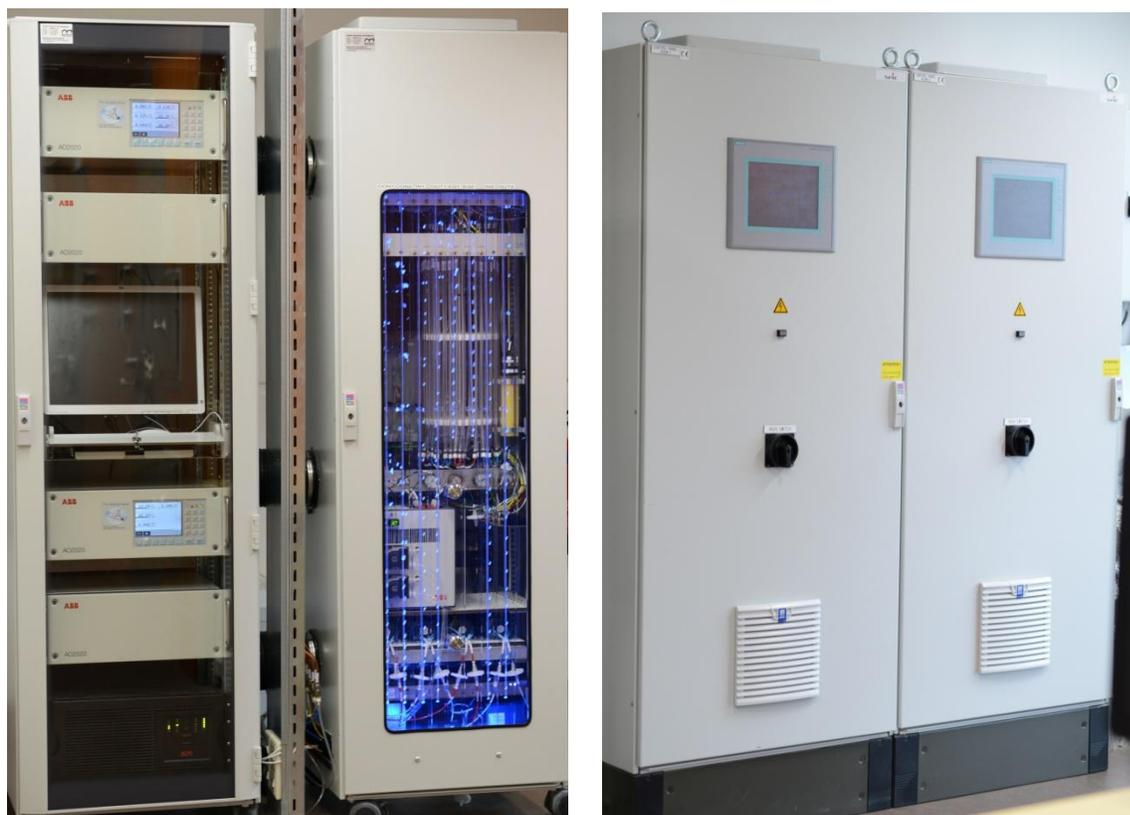
Fig 2.1. Gas processing and analysis units linked to a data acquisition computer
